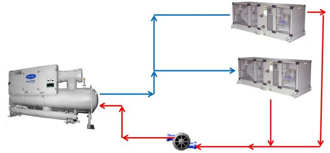
Figure 2- Simple Chilled Water Loop
