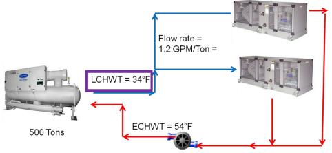
Figure 5 - Reduction in Flow Transient
