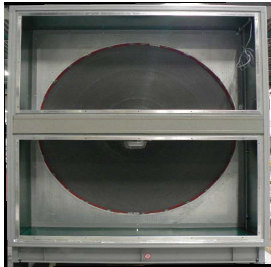
Heat Recovery Wheel
