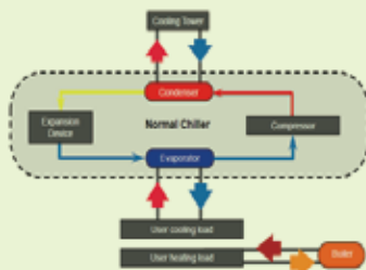
Traditional water-cooled chiller and boiler
